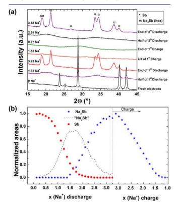
**Figure 4.** (a) Selected operando XRD patterns at various stages of discharge and charge of a Sb/Na cell. \*, and r were used to indicate the Bragg peaks corresponding to Sb and Na<sub>3</sub>Sb, respectively. (b) Normalized areas under the most intense diffraction peaks for Sb (28.8°) (in red) and Na<sub>3</sub>Sb (21.2°) (in blue) during the first cycle plotted as a function of Na number (*x*). The dashed line represents the calculated intensity of amorphous Na<sub>3</sub>Sb phase.
