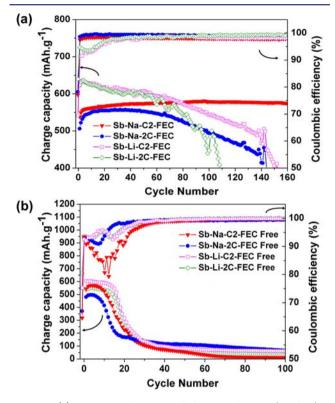
Figure 5. (a) Cycling performance of Sb electrode vs Na<sup>+</sup> and Li<sup>+</sup> at C/2 and 2C with (top) and (b) without (bottom) addition of 5% FEC.
