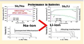
Sb/Na cell between the formation of the hexagonal and the cubic polymorphs of  $Na_3Sb$ , the last being described in the literature as unstable at atmospheric pressure and only synthesized under high pressure (1–9 GPa). In addition, fluoroethylene carbonate added to the electrolyte combined with an appropriate electrode formulation based on carboxymethyl cellulose, carbon black, and vapor ground carbon fibers seems to be determinant in the excellent performances of this material.
