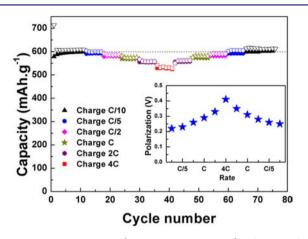
Figure 6. Rate capability (and polarization, inset) of the Sb/Na electrode at various current rates from C/10 to 4C. Open and filled symbols are for discharge and charge, respectively.
