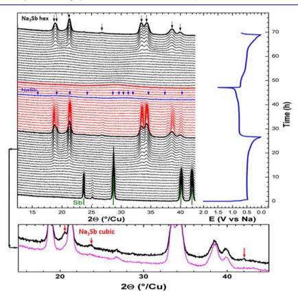
Figure 3. Operando evolution of the XRD pattern recorded at a C/8 rate (top left). The black and the red patterns are those recorded during the discharges and charge, respectively. The corresponding voltage profile (top right). A zoom illustrating the diffraction peaks from the cubic  $Na_3Sb$  (bottom).
